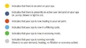
The widget on the home page displays a single color at a time. The color displayed is decided by priority of state. The established priority is as listed above.
