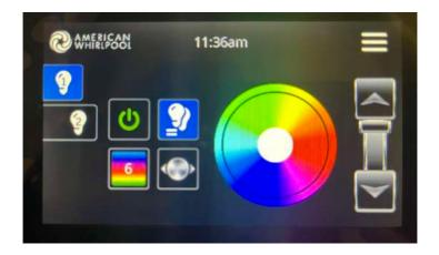
By default, in.mix selects Zone 1 when you access the menu. To lock both zones together, press the button with the two light bulbs. To unlock the two zones, press the same button again. Otherwise, adjust each zone by selecting the appropriate number on the left hand side.
